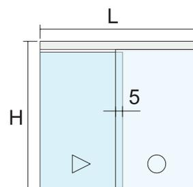
$$\begin{aligned} C &= (L/2) + 25\text{mm} \\ H_p &= H - 70\text{mm} \\ F &= (L/2) + 25\text{mm} \\ F_x &= H - 15\text{mm} \end{aligned}$$
